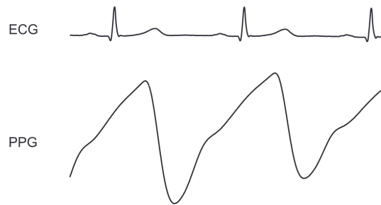
Figure 2.2: The PPG signal compared to the corresponding ECG recording of the HR. Adapted from Allen et al. [6].
